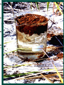
Floating bleaching earth/acid sludge depositions
